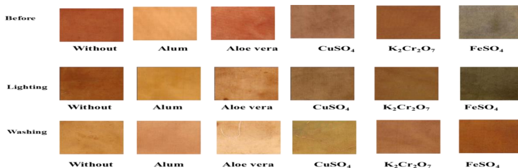
Figure 5. Variation in colour of Lining cloths after fastness test (Post mordanting )
