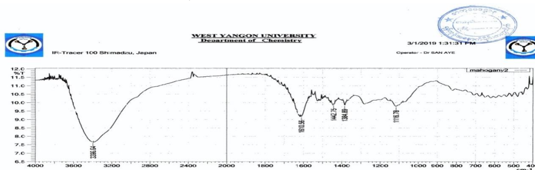
Figure 1. FT IR spectrum of natural dye extracted from Swietenia macrophylla King (Mahogany) barks
