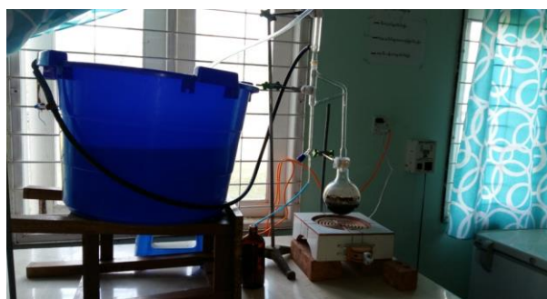
Figure 2. Extraction of essential oil from Eucalyptus leaves
