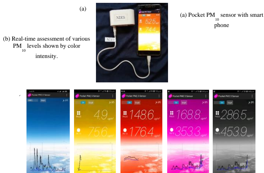
Fig. 2 Description of PM 10 Sensor
